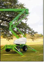
The extra manoeuvrability available from the 4 wheel steer option coupled with the special "Turf Tyres" make the **210SD** ideal for working on sensitive surfaces such as grass.
